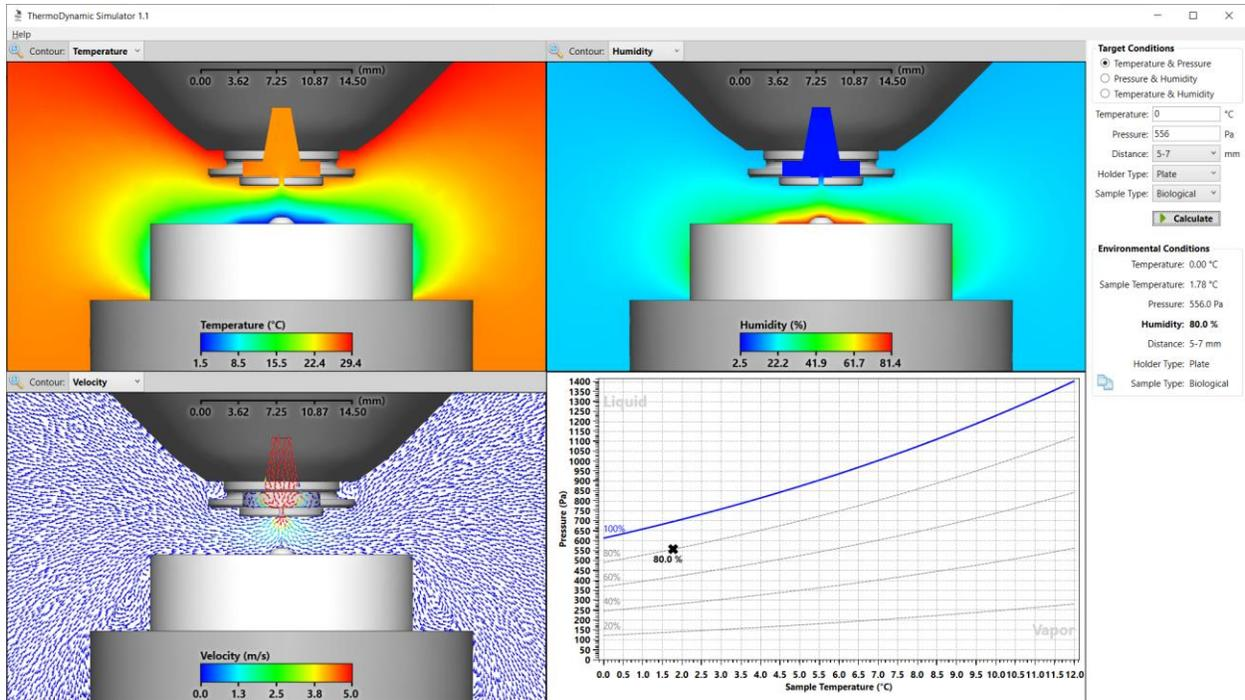
The testing procedures have shown that the TDS results are correlated with the measurements up to 3.5% of deviation.
